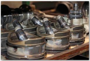
The most critical part on aircraft engine is without doubt the cylinder section. This part of the engine is exposed to stress, extreme temperatures, pressures, mechanical wear, chemicals and corrosion and often misuse by the operator as well.
